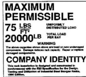
Example of a required load capacity and compliance plaque
